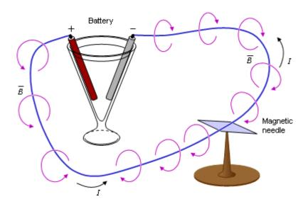
**Fig. 1.12.** Reconstruction of the first demonstration of the electromagnetic connection by Hans Christian Örsted in 1819. The battery generates an electric current I to flow in the circuit formed by a metal wire. This current induces a magnetic induction around the wire. The magnetic needle under the wire turns parallel to the direction of the magnetic induction demonstrating its existence. (Örsted, 1820a,b,c).
