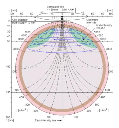
**Fig. 22.3** Iso-intensity lines (dashed black), induced stimulation currrent lines (solid blue) and half-intensity volume (green) for a stimulation coil with 50 mm radius. The distance of the coil plane from the scalp is 10 mm.
