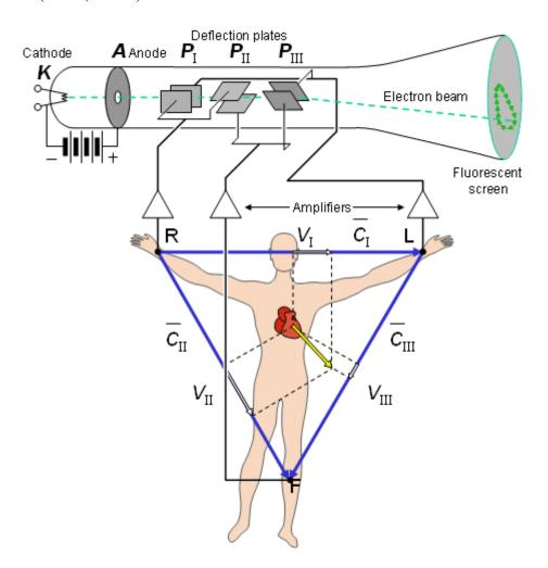
**Fig. 16.3** The cathode ray tube of W. Hollman and H. F. Hollman has three pairs of deflection plates oriented in the directions of the edges of the Einthoven triangle. Thus it produces the vectorcardiogram in the frontal plane from the Einthoven limb leads. (Hollman and Hollman, 1937)
