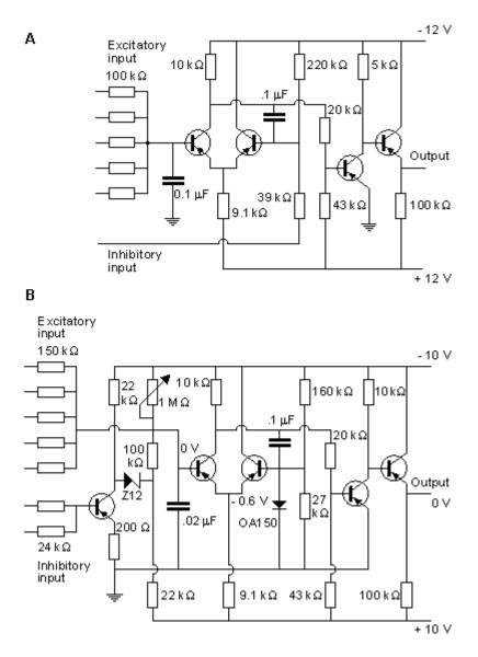
**Fig. 10.13.** Construction of the Harmon neuron model. (A) The preliminary and (B) the more advanced version of the circuit. Without external circuits, Harmon investigated successfully seven properties of his neuron model. These are illustrated in Figure 10.14 and are described briefly in the following.
