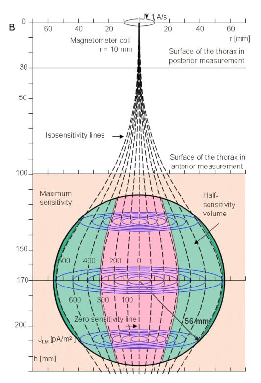
**Fig. 20.16** Sensitivity distribution of a bipolar (symmetric) measurement within the region of the spherical heart model. The figure also illustrates the anterior magnetometer. This measurement situation corresponds to the measurement of the x component of the MHV with the symmetric XYZ lead system or with the symmetric unipositional lead system with measurements on both sides of the thorax.
