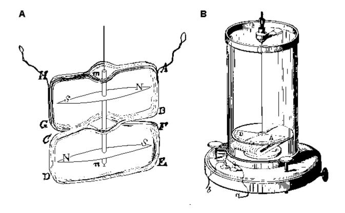
**Fig. 1.13.** (A) Astatic galvanometer invented by Nobili in 1825. He compensated for the effect of the Earth's magnetic field by placing two identical magnetic needles connected on the same suspension in opposite directions in the openings of a coil wound in the form of figure eight. (Nobili, 1825.) (B) A technically more advanced version of the astatic galvanometer. Only one of the two identical (but opposite) needles is surrounded by a coil. The other needle serves as an indicator.
