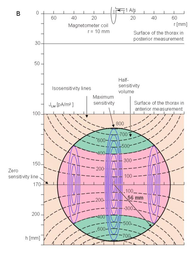
**Fig. 20.17** Sensitivity distribution in the measurement of the *y* component with the symmetric unipositional lead system illustrated (A) in the *zx* plane and (B) in the *yz* plane. Isosensitivity lines are illustrated with black dashed lines. Lead field current flow lines are sketched with blue solid lines.
