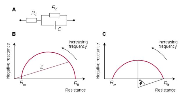
Fig. 25.1 (A) Three-element model of tissue impedance exhibiting a single time constant.
