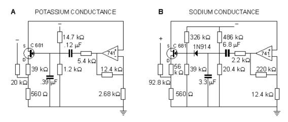
Fig. 10.6. The circuits simulating (A) sodium and (B) potassium conductances in the Roy membrane model.
