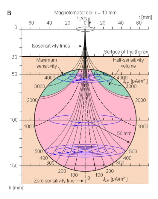
**Fig. 20.14** Sensitivity distribution of a unipolar (nonsymmetric) measurement within the region of the spherical heart model for a 100 mm magnetometer - heart center separation. The figure also illustrates the location and size of the magnetometer. This measurement situation corresponds to the measurement of the *x* component of the MHV with the nonsymmetric unipositional lead system in the anterior side of the thorax.
