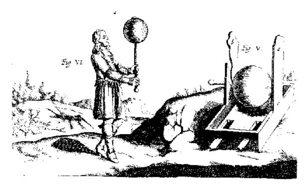
**Fig. 1.6.** Otto von Guericke constructed the first electric machine which included a sphere of sulphur with an iron axle. When rotating and rubbing the sphere it generated static electricity. (Guericke, 1672).
