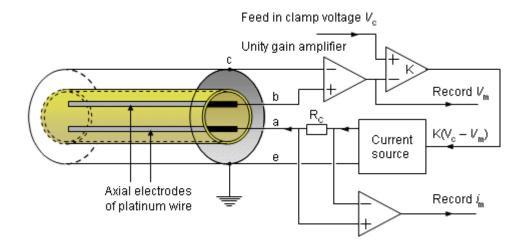
**Fig. 4.4.** Realistic voltage clamp measurement circuit. Current is applied through electrodes (a) and (e), while the transmembrane voltage,  $V_{\rm m}$ , is measured with electrodes (b) and (c). The current source is controlled to maintain the membrane voltage at some preselected value  $V_{\rm c}$ .
