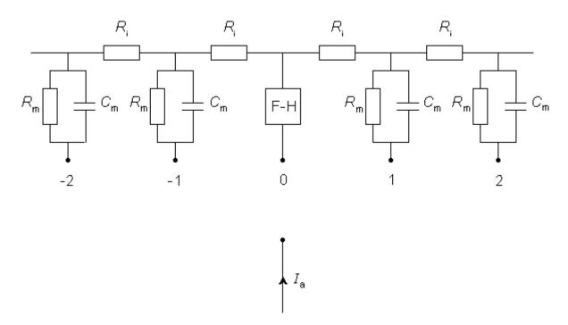
**Fig. 21.2** Electric model of a myelinated fiber stimulated by a point current source of strength  $I_a$ . The node directly beneath the source is labeled 0 and its membrane is modeled by Frankenhauser-Huxley (F-H) equations. Lateral nodes are assumed to be subthreshold and represented by parallel resistance and capacitance (where  $R_m$ ,  $C_m$  are the total nodal lumped resistance and capacitance per nodal area). The total intracellular internodal resistance is  $r_i$ .
