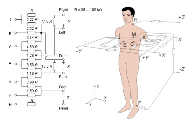
**Fig. 16.11** The lead matrix of the Frank VCG-system. The electrodes are marked I, E, C, A, M, F, and H, and their anatomical positions are shown. The resistor matrix results in the establishment of normalized *x*-, *y*-, and *z*-component lead vectors, as described in the text.
