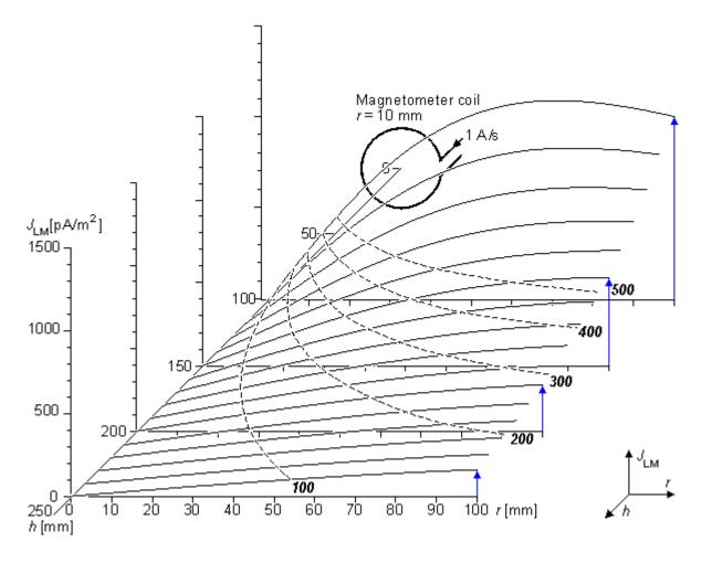
**Fig. 12.15.** The lead field current density distribution of a unipolar single-coil magnetometer with a 10 mm coil radius in a cylindrically symmetric volume conductor calculated from Equation 12.42. The dashed lines are the *isosensitivity lines*, joining the points where the lead field current density is 100, 200, 300, 400, and 500 pA/m<sup>2</sup>, respectively, as indicated by the numbers in italics.
