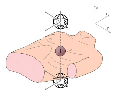
Fig. 20.12 Realization of the symmetric unipositional lead system.
