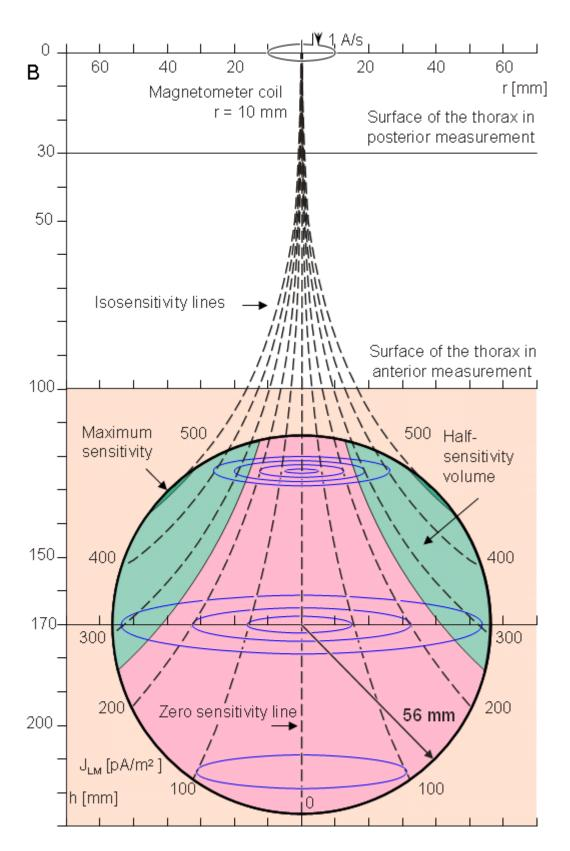
**Fig. 20.15** The sensitivity distribution of a unipolar (nonsymmetric) measurement within the region of the spherical heart model for a 170 mm magnetometer - heart center separation. This measurement situation corresponds to the measurement of the x component of the MHV at the posterior side of the thorax.
