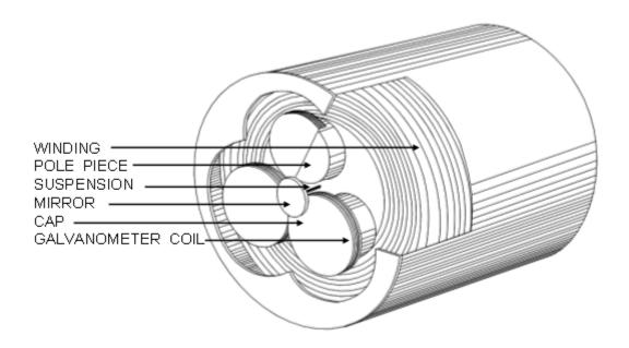
**Fig. 16.2** The mirror vectorcardiograph constructed by Hubert Mann was the first instrument to produce a vectorcardiogram. It has three coils symmetrically placed at 120° intervals around a mirror. Thus it produces a vectorcardiogram in the frontal plane from the three limb leads of Einthoven. (Mann, 1938a).
