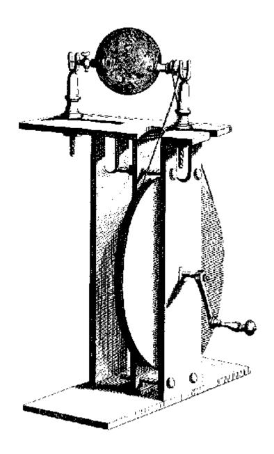
**Fig. 1.7.** Electric machine invented by Hauksbee in 1704. It had a sphere of glass rotated by a wheel. When the glass was rotated and rubbed it produced electricity continuously. If the glass was evacuated with air pump it generated brilliant light. (Hauksbee, 1709).
