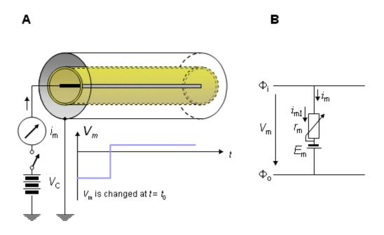
Fig. 4.3. Voltage clamp experiment.
