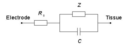
**Figure 21.10** The electrode-tissue interface includes a series ohmic resistance Rs, a series capacitance Cs, and a Faradaic impedance Z. The capacitance represents a double layer that arises at the metal-electrolyte interface, whereas the Faradaic impedance includes several physical and chemical processes that may occur.
