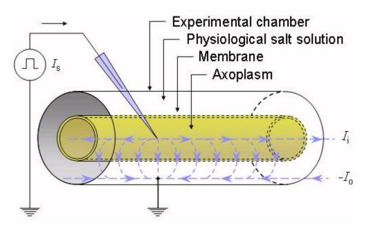
Fig. 3.6. The experimental arrangement for deriving the cable equation of the axon.
