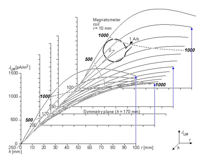
**Fig. 12.19.** The lead field current density distribution of a bipolar lead in a cylindrically symmetric volume conductor realized with two coaxial single-coil magnetometers with 10 mm coil radius. The distance between the coils is 340 mm. The dashed lines are the *isosensitivity lines*, joining the points where the lead field current density is 500 and 1000 pA/m<sup>2</sup>, respectively, as indicated with the numbers in italics.
