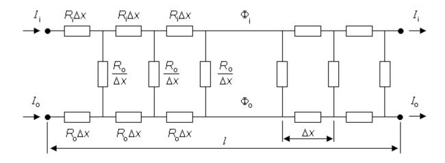
**Fig. 24.4** Core-conductor electric network for a single cell that is a component of an equivalent single cardiac fiber. The cell is connected to its neighbors by an intracellular coupling resistance, Rj, at its ends. Steady-state subthreshold conditions are assumed.
