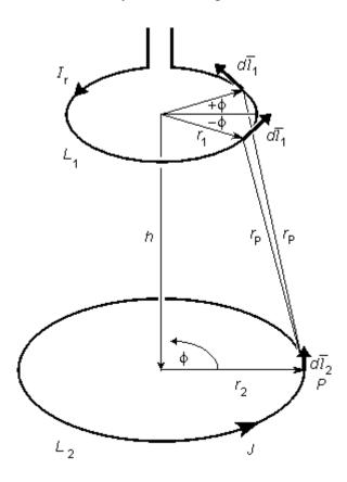
**Fig. 12.14.** Geometry for calculating the spatial sensitivity of a magnetometer in a cylindrically symmetric situation.
