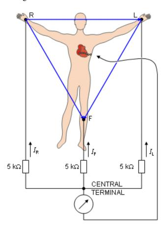
**Fig. 15.5.** The Wilson central terminal (CT) is formed by connecting a 5 kΩ resistance to each limb electrode and interconnecting the free wires; the CT is the common point. The Wilson central terminal represents the average of the limb potentials. Because no current flows through a high-impedance voltmeter, Kirchhoff's law requires that  $I_R + I_L + I_F = 0$ .
