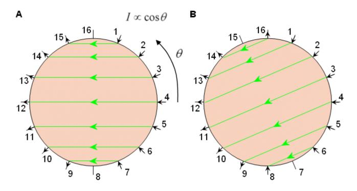
Fig. 26.4 Adaptive method of impedance data collection.
