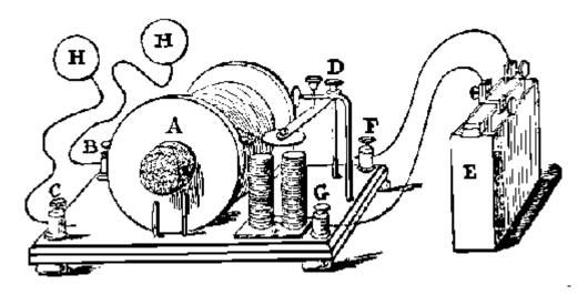
**Fig. 1.10.** Induction coil with hammer break. Electric current from the battery (E) is fed to the primary circuit of the induction coil (A). This current pulls the hammer with the magnetic field of the solenoid (close to G) and breaks the circuit with the contactor (D). Through the vibration of the hammer this breaking is continuous and it induces a high voltage alternating current in the secondary circuit in (A). This current is applied to the patient with electrodes (H)..
