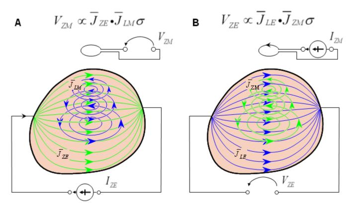
Fig. 26.5 Electromagnetic method of impedance data collection.
