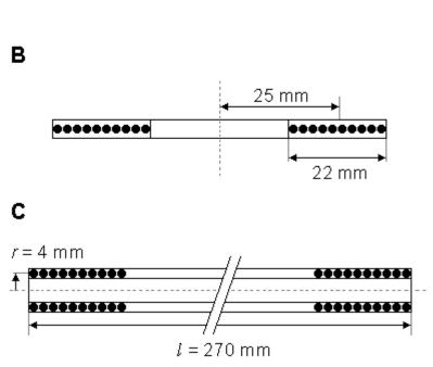
Fig. 22.2 Dimensions of coils of different configuration:
