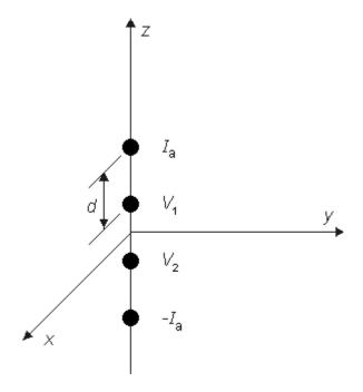
**Figure 9.5.** Four-electrode method for the determination of tissue impedance. The electrode is embedded in the tissue. The outer elements carry the applied current  $\pm I_a$  while the inner elements measure the resulting voltage  $(V_Z = V_1 - V_2)$ . The electrodes are spaced a distance (a) from each other (equispaced). For a uniform isotropic monodomain, the resistivity  $\rho = 2\pi dV_Z/I_a$ .
