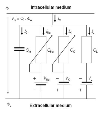
**Fig. 3.4.** An electric circuit representation of a membrane patch. In this diagram,  $V_{\text{Na}}$ ,  $V_{\text{K}}$ , and  $V_{\text{L}}$  represent the absolute values of the respective emf's and the signs indicate their directions when the extracellular medium has a normal composition (high Na and Cl, and low K, concentrations).
